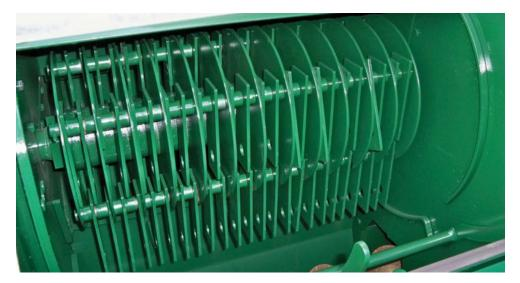
26 inch one-piece hammermill design with 96 4-way reversible knives. Provides a more consistent grind for improved feed rations. Exceptional grinding capacity.
