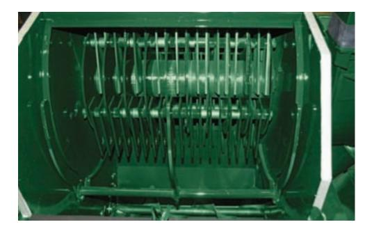
20 inch one-piece hammermill design with 72 4-way reversible knives. Provides a more consistent grind for improved feed rations. Exceptional grinding capacity.
