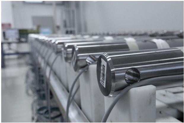
Production Testing. Dinamica Generale load cell undergoes many accuracy tests followed by stress tests prior to production completion. These standard procedures help prevent product defect before they arise and at the same time build trust and loyalty with customers.
